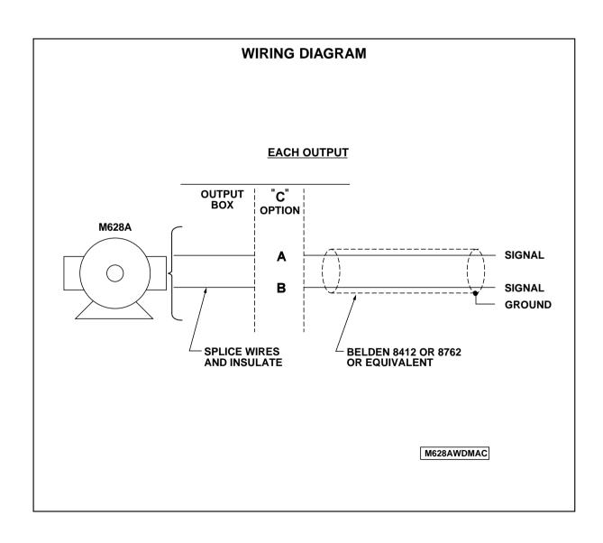
NOTE: OUTPUT CONNECTORS ARE SHOWN FACING DOWN FOR CLARITY. CONNECTORS WILL BE POSITIONED TOWARDS "C" FACE FOR SHIPMENT FROM FACTORY.
